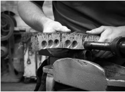
Bottle corks are punched out of sections of prepared bark ready for their new use.
